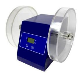
The microprocessor-controlled Friability Tester allows programming of a specific time interval or set number / number of turns.
